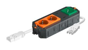
The ready-for-connection UTC4 universal support has 2 pre-installed 33° protective contact sockets in orange and one pre-installed 33° protective contact socket in mint green and one blanking cover for retroinstallation of an installation device of the Modul 45 or Modul 45connect series, 250 V $\sim$ , 16 A.
