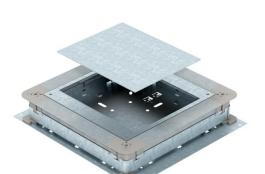
Underfloor accessory box for screed-covered underfloor installation ducts with sheet steel side walls. To mount installation units of the selected nominal size. Height can be infinitely adjusted to the nominal screed height (rapid adjustment possible) and the screed can be worked flush to the screed scraping edge. With noise decoupling option after screed laying and can be used with system accessories, also for heavy-duty application.
