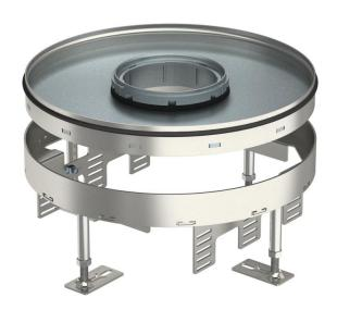
Round heavy-duty cassette for tube body of nominal size R9 for the installation of accessories in trunking systems, raised and cavity floors, in dry or wet-cleaned floors. Load class 2 to 20 kN.
