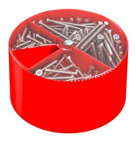
Set consisting of 100 device screws each of types KGS 15, 25 and 40 for device and lid fastening, with self-tapping thread  $\varnothing$  3.2 mm. Including storage box with separate compartments for the different screw types,  $\varnothing$  95 x 55 mm.
