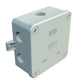
Protection rating IP67, empty box for use with individual terminals, four plastic cover screws, thus absolute corrosion-protection, two fastening bases for screws of up to 5 mm Ø, 7 break-out entries with thread M20 x 1.5. 3 polyamide cable glands for cable diameters of 9–12 mm, type 106 M.
