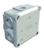
Protection rating IP54, rated voltage 660 V, nominal cross-section 2.5  $\div$  4, in combination with the earthing terminal 700/6 M, the box has the nominal crosssection 4 mm², two fastening holes for screws of up to 5 mm  $\varnothing$  on the outer side of the box. Four cover screws, 7 break-out entries with thread M20 x 1.5, primarily for cable glands with short connecting thread.
