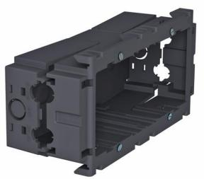
Front locking accessory mounting box for standard switch ranges for the installation of two individual installation devices or a multiple protective contact socket. With unfolding, and also removable, base for time-saving cable connection and with feed openings for cable diameters of up to 14 mm. Halogen-free version. Vertical fixing track 60 mm.
